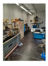
The shed has seen great improvements and expansion in the last month. through purchases and donations we have acquired a metal lathe, a drill press and mill, a saw and steel cutter, a metal folder, a steel work table, two welders, and a steel accessory cupboard, among other things.
